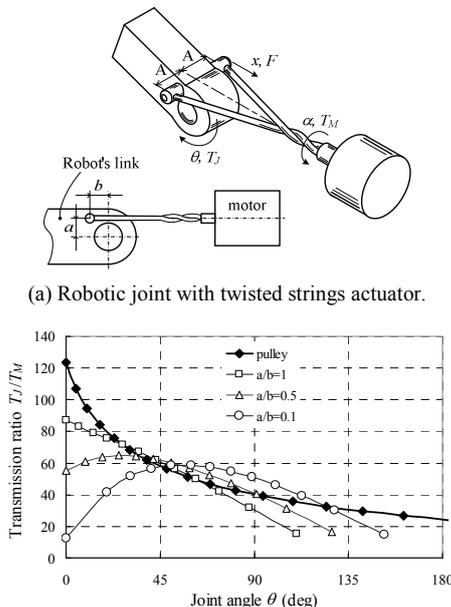
(b) Transmission characteristic for different configurations.
