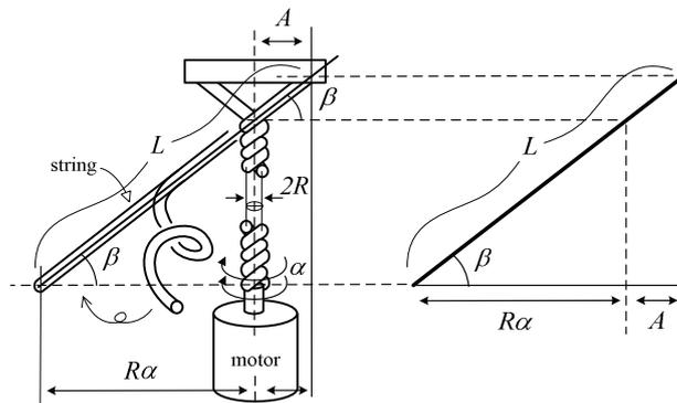
Figure 1. Twisted strings actuation principle.
