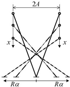
Figure 2. Geometrical representation of twisted strings actuation.
